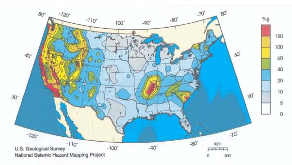
Figure 9a. MCE ground motion map of the 48 conterminous states for the 0.2 sec horizontal spectral response acceleration (%g), 5% of critical damping, Site Class B.
