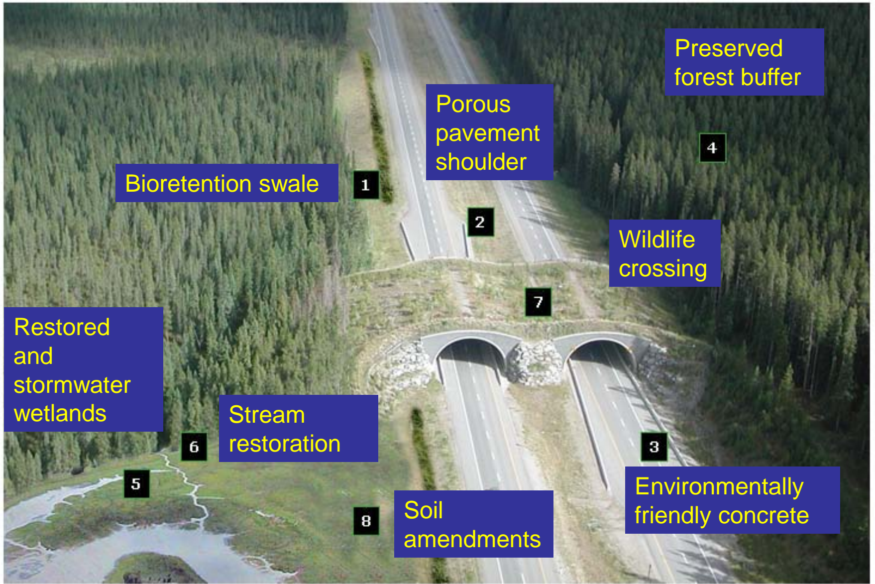
This picture has been edited from its original format to illustrate Green Highways technologies. Original photograph taken by Tony Clevenger.
