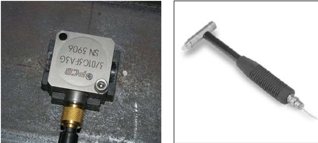
Figure 4-14 PCB capacitive accelerometer model 3701G3FA3G (left) and PCB impulse-force test hammer model 086C02 (right)
