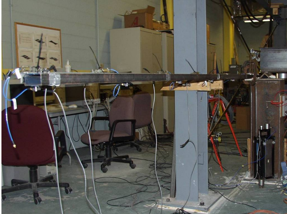
Figure 4-9 Test beam setup 1 with fixed support
