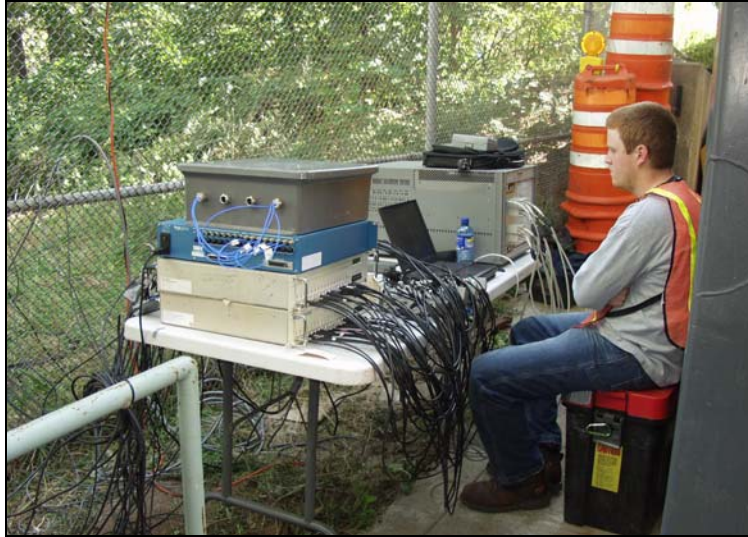
Figure 5-13 Data acquisition system at the Henry Hudson Bri
