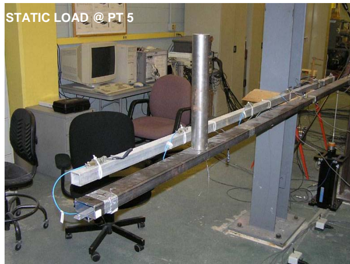
Figure 4-24 Static test on the cantilever beam
